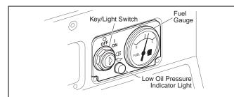
Fig. 9 Key/Light Switch, Low Oil Pressure Light and Fuel Gauge
